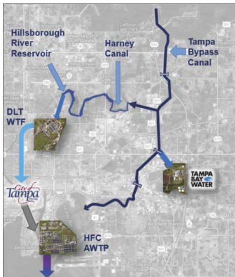
Figure 2. Regional potable water supply system considered in the Tampa Augmentation Project.
